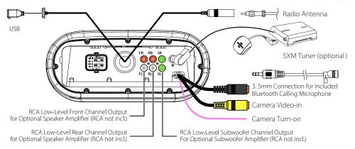
6. Take a moment to reinstall the main fuse if it was removed. At this point, HDHU.9813RG should turnon. Verify all speakers are playing and the head unit is functioning. If successful, tie any loose wires that might impede reinstallation of the fairing.
