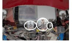
6. Gently pull the OEM radio out and up, away from the support bracket. No other parts from the OEM radio are needed.
