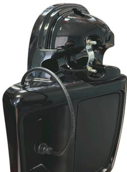
**Tip:** Use a small/mini flathead screwdriver to press one side of the rubber grommet thru the fairing sidewall.
