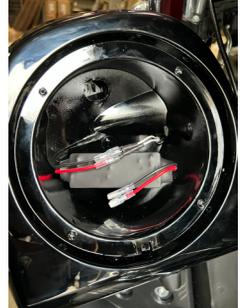
3. Connect the FEMALE terminals of the EQ module to the corresponding MALE terminals of the speaker. Red wire to + terminal of the speaker, black wire to the – terminal of the speaker.
