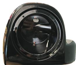
**Tip:** Insert one speaker terminal at a time thru the hole in the speaker pod. If the hole is too small, use a 1/4" drill bit & cordless drill to enlarge the hole.
