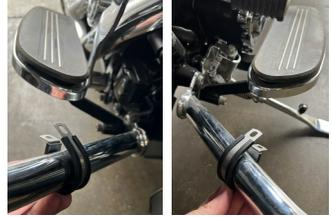
8. With one hand, hold the lower fairing assembly in place to the crash bar, aligning the upper portion of the crash bar into the crash bar channel of the lower fairing. With another hand, join the crash bar cover removed in #2 to the lower fairing.
