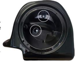
3. Flip the fairings over and remove the three Phillips screws to release the speaker pod. Set the speaker pods & screws aside.
