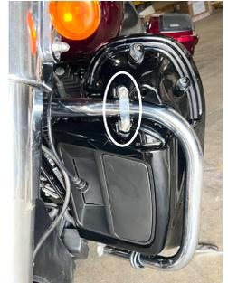
10. Align the screw hole of the lower crash bar clamp to the hole in the bottom of the lower fairing. Push a lower crash bar clamp hex bolt with washer included in the kit thru the hole in the lower portion of the fairing and thru the holes of the lower crash bar clamp installed in step 8.
