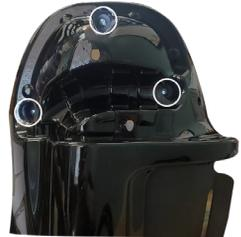
4. Thread the speaker wire included with this kit thru a hole in the sidewall of the lower fairing, located near the crash bar channel. Insert the speaker wire terminals first, pulling about 6" of speaker wire into the fairing. Insert one side of the rubber grommet thru the hole into the fairing.
