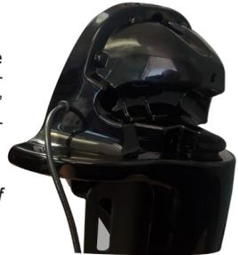
5. Thread the speaker wire thru a hole in the back of the speaker pod removed in step #3. Leave about 3" of speaker wire inside the speaker pod, and 3" between speaker pod and the lower fairing.
