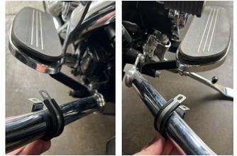
9. With one hand, hold the lower fairing assembly in place to the crash bar, aligning the upper portion of the crash bar into the crash bar channel of the lower fairing. With your third & fourth hands (or a helper), reattach the upper crash bar clamp using a ratchet & 10mm socket on an extension. Secure only hand tight so final adjustments can be made later.
