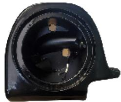
6. Hold the speaker pod and fairing together and flip the assembly over, aligning the screw holes of the speaker pod to the lower fairing. Reattach the speaker pod to the lower fairing using the three Phillips screws removed in step 3. Set the complete speaker pod & lower fairing assembly aside.
