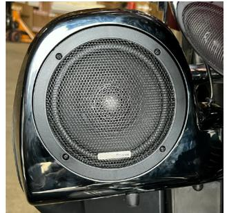
5. Align the speaker/grill assembly with screws to the screw holes of the speaker pod. Attach the grill & speaker to the speaker/grill assembly to the pod using a #2 phillips screwdriver.
