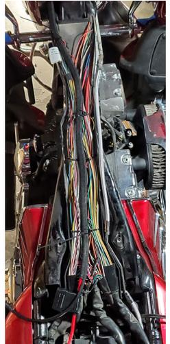
2. Connect the threaded connector end of the backbone cable to the T-connector input. Route the backbone cable in the wire chase and speaker output connector end thru the fairing to the amplifier location. Use cable ties to loosely secure the backbone cable to adjacent cables in the fairing & wire chase.
