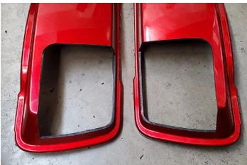
5. Following the traced cut-out lines, cut away the speaker opening from each lid. If using a jig-saw or air-saw, pre-drill a 3/8" hole within the cut-out area to accommodate the start of your cut. After the center section has been cut away, use a metal file to smooth-out any rough edges and corners. **SAFETY GLASSES ARE A MUST!!!!**
