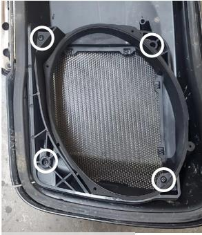
6. While holding the grill in place on the top surface of the lid, turn the lid over and line-up the speaker adapter screw holes. Use four small headed phillips screws provided to attach the speaker adapter to the grill.
