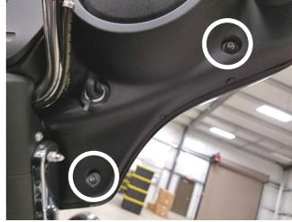
3. While straddling the front wheel fender, grasp the outer fairing, remove the center outer fairing bolt from the previous step, then gently pull the fairing apart from the bike. With the fairing slightly pulled away from the bike, disconnect wire harness for the headlamp and any other accessories. Lay the fairing on a protected flat surface to prevent damage.
