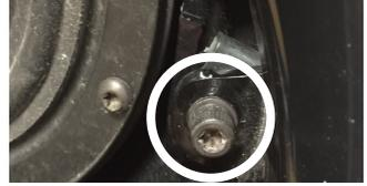
6. While straddling the front wheel fender, grasp the outer fairing. Gently pull the fairing apart from the bike. With the fairing slightly pulled away from the bike, disconnect wire harness for the headlamp or any other accessories. Lay the fairing on a protected flat surface to prevent damage.
