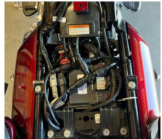
6. Connect each saddlebag speaker cable to its corresponding side of the T-connector. Brake side saddlebag speaker cable connects to the “Lch.” side of the T-connector, and brake side saddlebag speaker cable connects to the “Rch” side.
