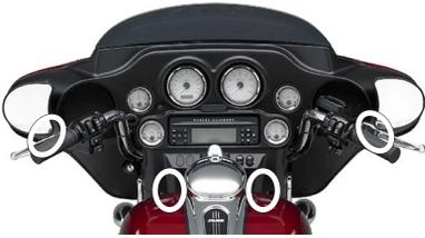
2. Remove four inner fairing bolts using a T27 Torx screw driver. Two inner fairing bolts are located adjacent to each mirror. Two additional screws are adjacent to the forks. Store these screws in a safe place for re-installation later.
