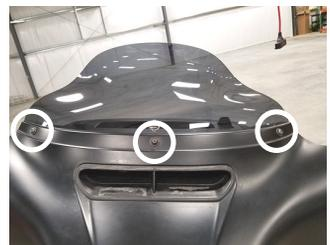
**TIP:** Reinstalling the center screw after removing the windshield will prevent the outer fairing from falling during the next step. A few turns by hand will be sufficient.
