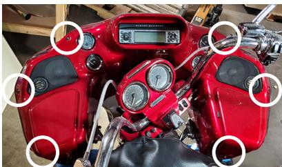
2. Remove six inner fairing bolts using a T25 Torx screw driver. Two screws are adjacent to the fuel & battery voltage gauges. Two more are located at the outside corner of each speaker grill. The last two screws are below each storage compartment hinge. Store these screws in the storage compartments for re-installation later.
