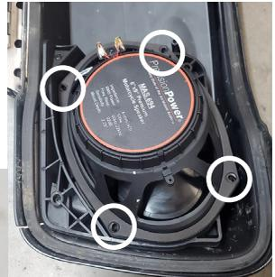
Attach the speaker using four large headed phillips screws provide.
