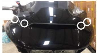
4. After removing the vent, locate and unplug the 3-pin wire harness for the left and right side turn signal indicator. These harnesses are adjacent to each side of the head unit.
