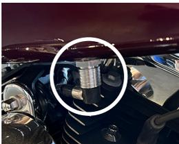
2. Disconnect the fuel line from the fuel tank by pressing up on the sleeve & gently pulling the line out.
