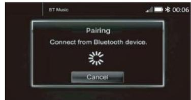
Turn on the Bluetooth of the Mobile phone/ Bluetooth device; you can see the "WHD14+." Select the "WHD14+" for pairing and connection.
