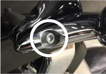
2. Remove four inner fairing bolts using a T25 Torx driver. Two inner fairing bolts are located below each glove box, adjacent to each wind deflector. Store these screws in a safe place for installation later.
