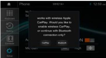
2. When the headunit detect the available device, follow the pop-up notice step by step to connect the iPhone. After connected, will show below page:
