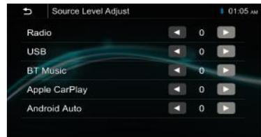
User can adjust the source mode (**Radio, USB, BT Audio, Apple CarPlay, Android Auto**) gain value. The gain can be adjusted from -5~+5 seperately.
