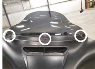
**TIP:** Reinstalling the center screw after removing the windshield will prevent the outer fairing from falling during the next step. A few turned by hand will be sufficient.
