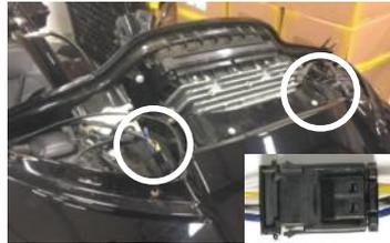
5. Remove an additional inner fairing bolt with a T27 Torx or 5/32" allen driver, one behind each speaker grill. Remove the speaker grill by wedging a plastic/nylon pry tool between the inner fairing and grill edge, popping it outward. Once these bolts are removed, the outer fairing will be detached from the inner fairing. Store these screws in a safe place for installation later.
